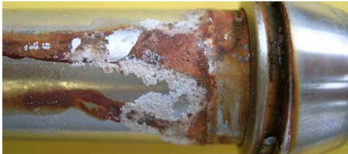
**Failure approaches — in just 7 days!** This image shows corrosion around a tube fitting assembly after just 175 hours exposure to salt spray (as per ASTM B117), a common problem in offshore environments. The tubing itself — also sourced from a low cost producer — is corroding just as rapidly.
